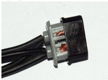
8) Slide on connector cap
