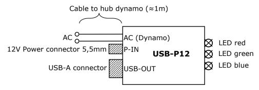
AC: input, connection to hub dynamo, two-core cable, 1m, black, fixed to box P-IN: Power connector (female) 5.5mm, input 12V, for usage with attached mains charger USB-OUT: output, USB-connector type A, 5V / 1A max.
