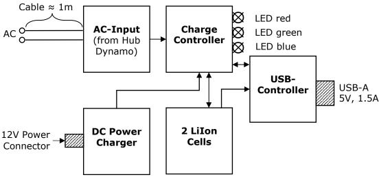
Fig. 2: Harvester Functional Diagram
