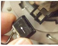
Disconnect and remember the wire which was connected to GND (symbol L\*\*)
