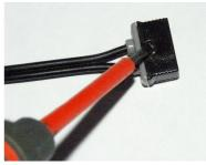
3) press flap with suitable tool (e.g. small screwdriver)
