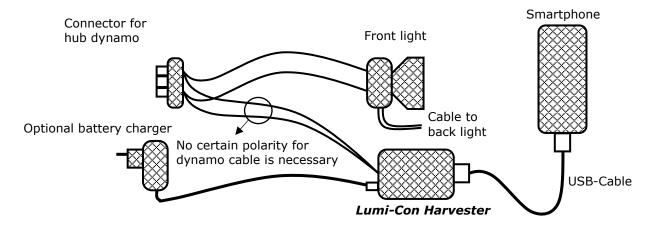
Fig. 6: Connecting the *Lumi-Con-Harvester*
