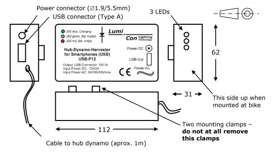
Fig. 5: Dimensions and Interfaces
